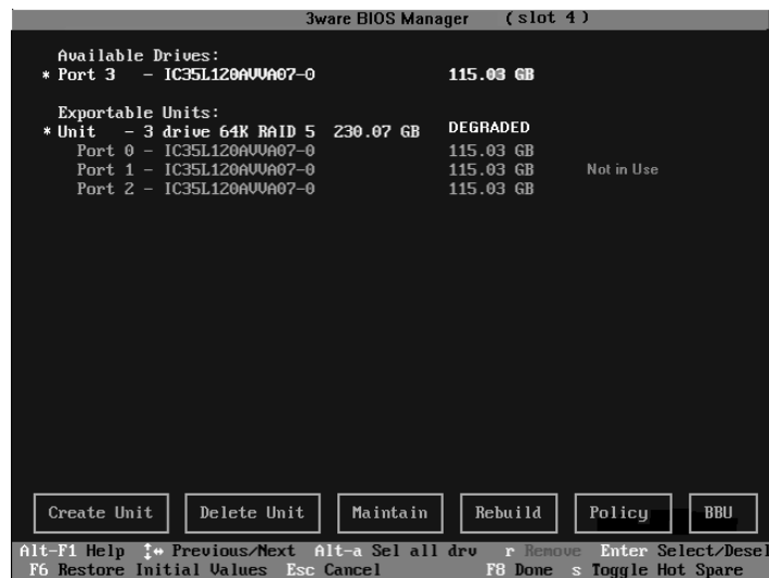
Figure 48. Select Available Drive to Replace Faulted Drive
