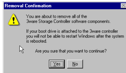
Figure 69. A Warning for All Software Removal Requests
